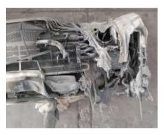
The initial sparks from the air conditioner in the above photo grew into a fire within two to three minutes. Molten plastic from the product's outer shell fell to the floor and continued to burn, resulting in an incident. According to an air conditioner technician, if the fire in the indoor unit had not been extinguished immediately, the refrigerant pipe would have ruptured, resulting in an explosion. This suggest that if this episode is unnoticed, it could have resulted in a massive disaster.
